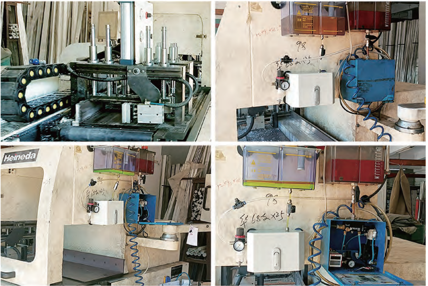
MQL on aluminum blanking machine
